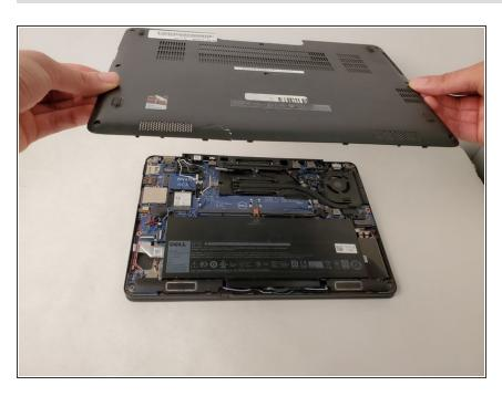
Lift and remove the panel.
