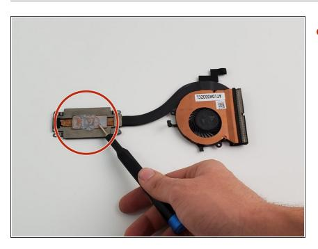
Before replacing fan, make sure to place a small amount of thermal paste to ensure proper heat dissipation and long term life.
