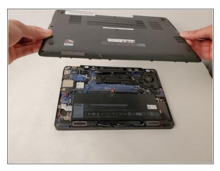
Lift and remove the panel.
