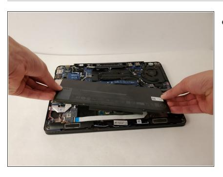
Remove the battery completely by grabbing an edge and pulling up on the battery.
