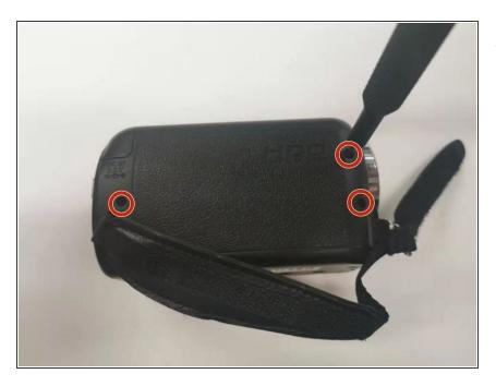
Remove three Phillips #00 screws from the left-hand side of the camera.
