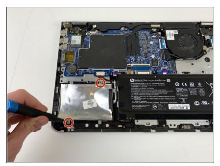
Remove the two 4.6 mm screws securing old hard drive/solid-state drive in place using the Phillips #0 screwdriver.
