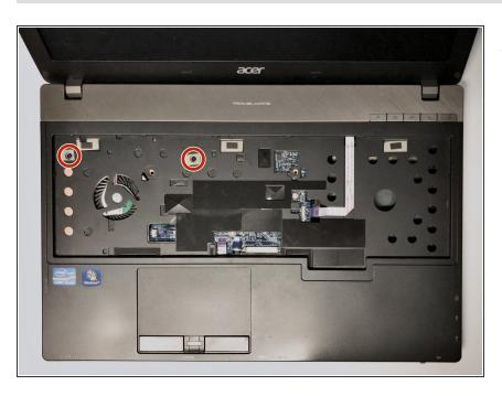
Using the #1 Phillips screwdriver, remove the two screws.
