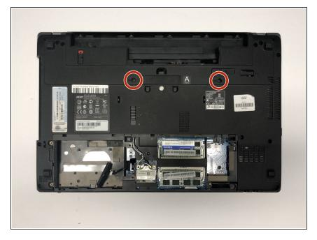
Remove the two 7mm Phillips #1 screws.
