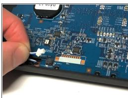
Disconnect the left speaker cable from the mainboard.
