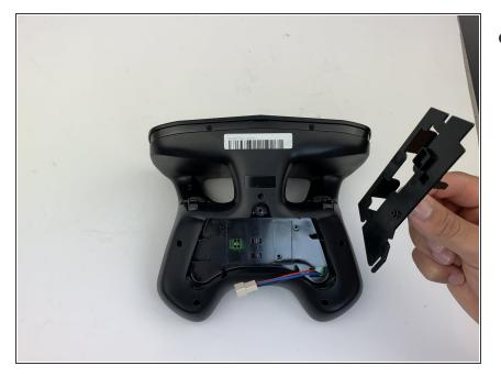
Remove the battery compartment plate by pulling up and out.
