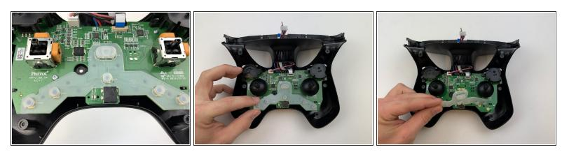
• Use some force pull up and out on the rubber backing for the buttons.
