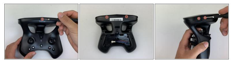
Remove the seven silver 4mm screws from around the edge of the top plate using the Torx TR6 Screwdriver.
