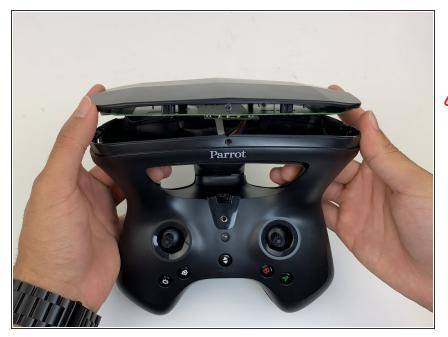
• Remove the top plate by pushing on the corners with your hand.
