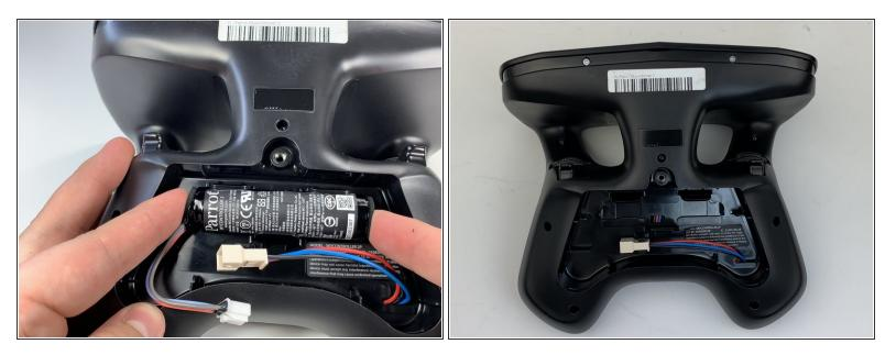
• Remove the battery from its brackets by pulling up on the ends of the battery.
