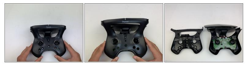
• Remove the face plate by pulling up and out.
