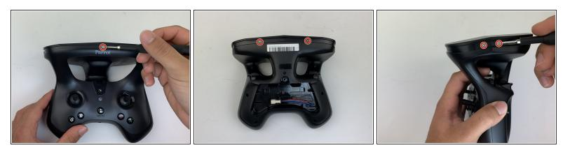
Remove the seven silver 4mm screws from around the edge of the top panel using the Torx TR6 Screwdriver.
