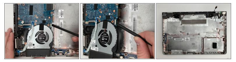
Using the plastic Spudger, gently lift up on the motherboard from the side that has the fan connected to it and remove the motherboard from the base.
