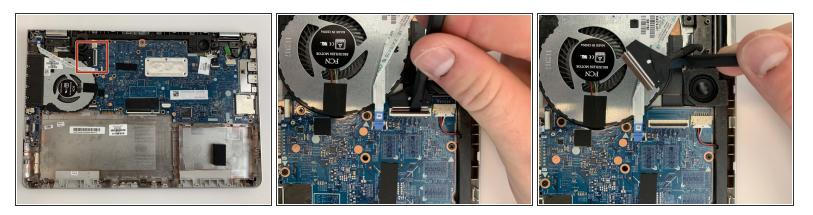
Using the plastic Spudger, remove the ZIF connector that connects the motherboard to the Display Cable. To remove a ZIF connector, use the flat end of the Spudger to flip up the cap on the top. Then the connector should slide out.
