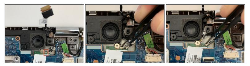
Use the Blunt Tweezers to disconnect the Wireless Card Antenna Cables. Start with the cable labeled M2, which is connected to Port #2. To disconnect he cable, grab it on both sides with the tweezers and pull up.
