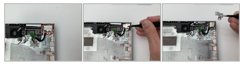
Using the Blunt Tweezers, gently lift the metal piece that covers the DC Power Jack unit and the metal piece will pop out.
