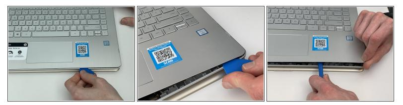
Using the iFixit Plastic Opening Tool and the iFixit Opening Picks, work your way around the rest of the keyboard and pry it out of the base.
