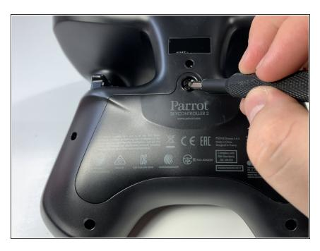
Remove one 9mm screw using a #4 flathead screwdriver.
