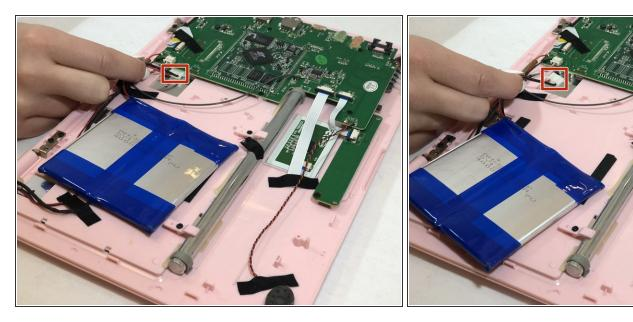
Pinch the red and black wires connected to the section closest to the small white connector, and pull to remove them from the motherboard. To reassemble your device, follow these instructions in reverse order.
