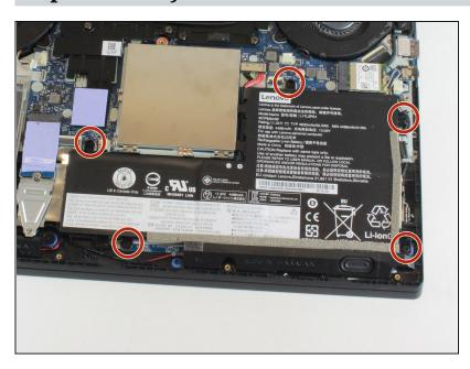
Use a Phillips screwdriver to remove the five 4 mm screws holding the battery in place.
