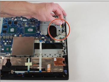
• Start by disconnecting the ribbon cable that is near the audio driver. It is recommended to use the iFixit Opening Pick to remove the ribbon cable.
