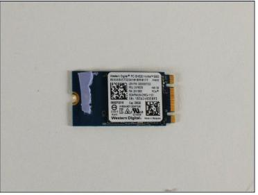
Carefully remove the SSD from its connector.
