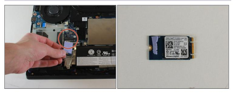
• Carefully remove the SSD from its connector.
