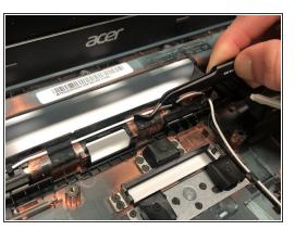
Carefully remove the two pieces of black tape securing the antenna cables to the lower case using tweezers.
