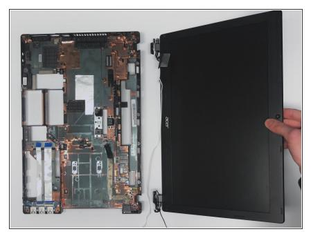
Carefully remove the LCD module from the lower case.
