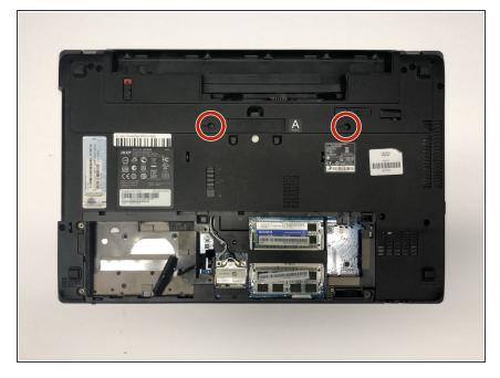
Remove the two 7mm Phillips #1 screws.
