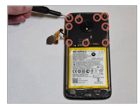
Remove the nine 3.2 mm screws from the motherboard cover with a Phillips #00 screwdriver.
