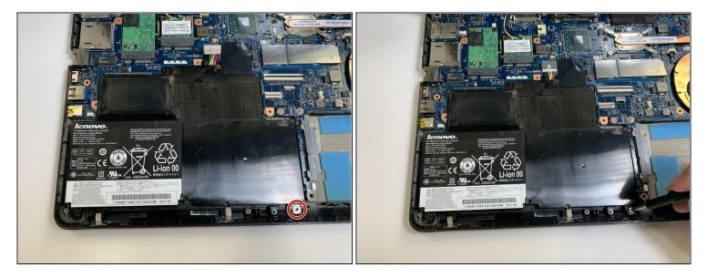
• Remove the single silver screw using the Phillips #1 screwdriver.
