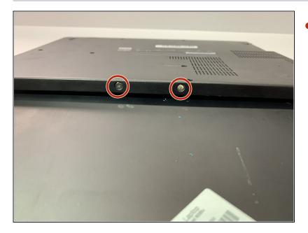
• Using the Phillips #0 screwdriver remove the two screws.
