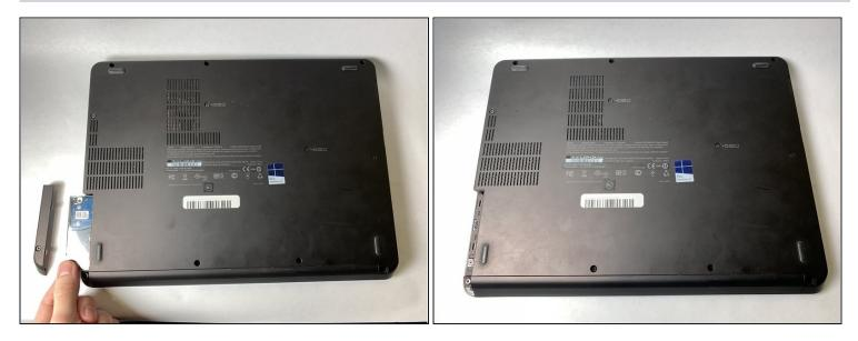
• Remove the hard drive by sliding it out.
