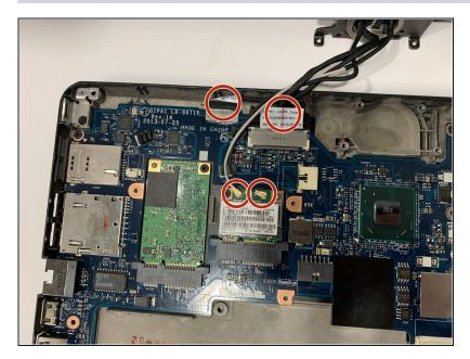
• Disconnect the four cables and remove the screen assembly from the device.
