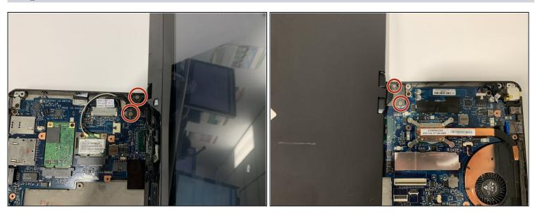
• Using the Phillips #1 screwdriver remove the four screws holding the screen to the laptop.
