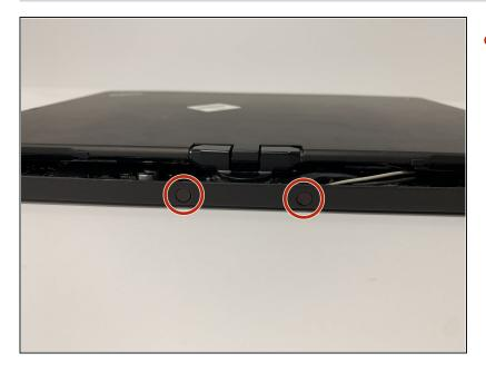
• Turn laptop around and remove the two screw covers.
