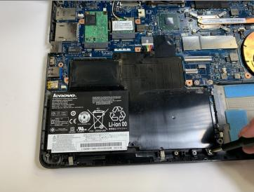
• Remove the single silver screw using the Phillips #1 screwdriver.
