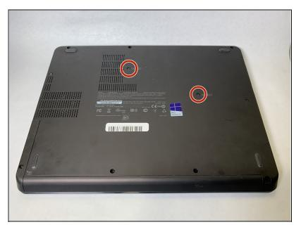
• Use a Philips #1 screwdriver to remove 2 screws on the bottom of the laptop.
