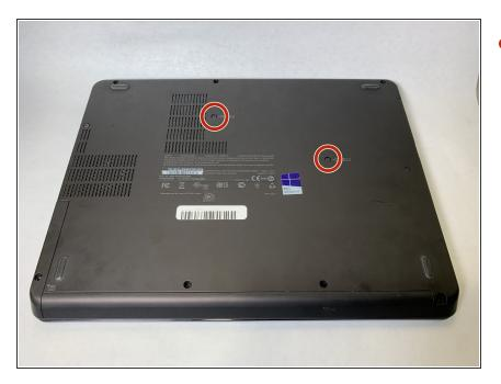
Use a Philips #1 screwdriver to remove 2 screws on the bottom of the laptop.
