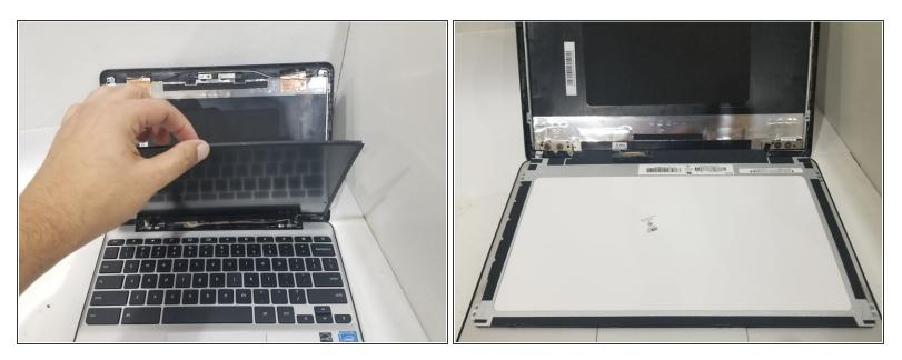
• Gently lift the LCD panel out of the body and lower it onto the keyboard deck.
