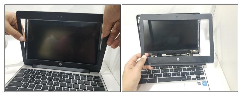
Hold the bezel on both sides, and twist the bezel repeatedly until the bottom bezel snaps out of place.
