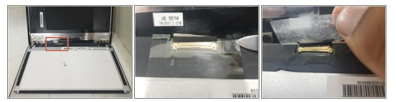
• Identify the eDP 30-pin connector and use the sharp end of the spudger to peel off a corner of the tape over the connector.
