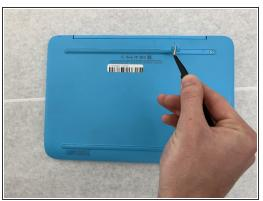
Gently peel back the two rubber strips that cover the screws on backside of the computer with the needle nose tweezers.
