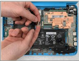
Use your fingers or a spudger to pull the battery cable out from its connector.
