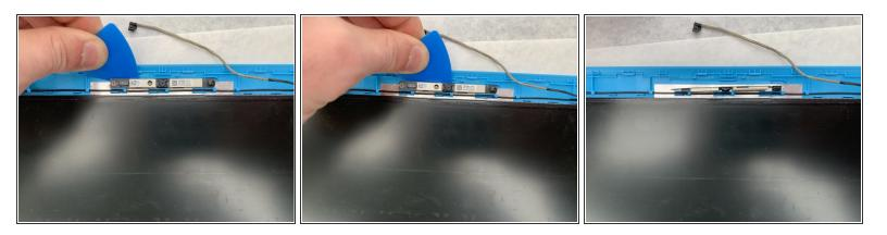
Take an iFixit opening pick and slowly remove the webcam by sliding it under the camera and prying the entire strip from the case.
