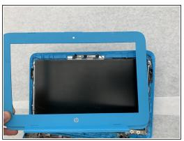
Remove the plastic bezel by pulling upwards on the bottom left corner.
