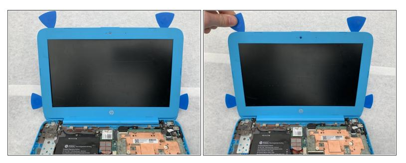
• Insert iFixit opening picks into the edges of the screen to break seal between the screen and bezel.
