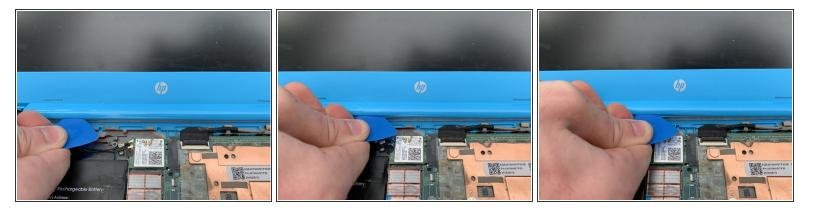
Peel the hinge up by sliding the iFixit opening picks left to right along the hinge.
