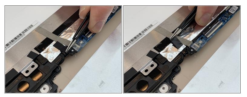
Using the Blunt Tweezers, remove the black tape covering the connection cable between the screen and the rest of the laptop.
