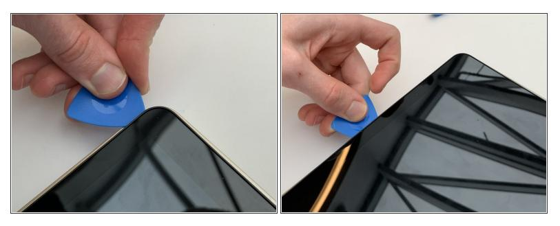
Once an initial separation between the casing and the screen has been made, use the iFixit Plastic
