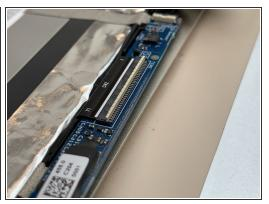
Using the flat end of a plastic Spudger, flip up the cap on the two ZIF connectors covering the gravity induction line and the touch line.
