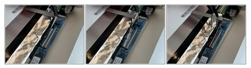
Using the Angled Tweezers, pull the ZIF connectors out of their housing.
