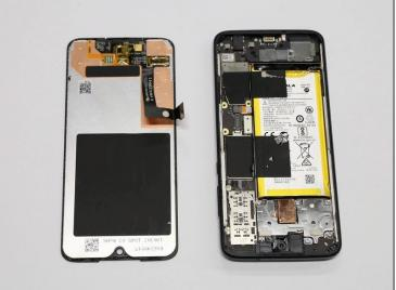
• Underneath this metal piece is the base of the cable. Use a spudger to vertically lift the connection out of its port.
