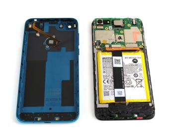
With the angled tweezers, detach the fingerprint scanner connector from the motherboard by pulling the metal head up and away from the phone.
