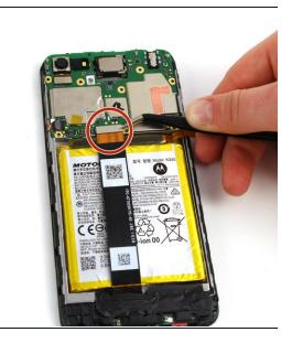
• With the angled tweezers, remove the horizontal and vertical connectors that link the battery to the motherboard together by pulling the metal heads on the connectors.
