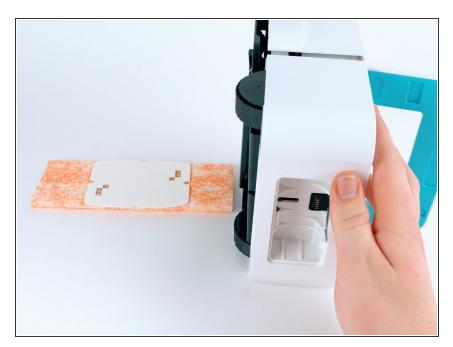
Tilt the robot on its side and let the mop pad slide out.
