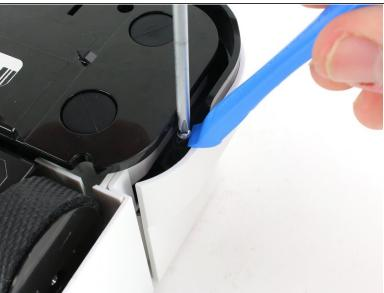
Use a Phillips #1 screwdriver and an iFixit opening tool to remove the two 15.0 mm screws on the front sides of the robot.
