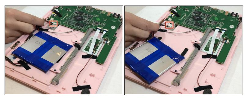
Pinch the red and black wires connected to the section closest to the small white connector, and pull to remove them from the motherboard.
