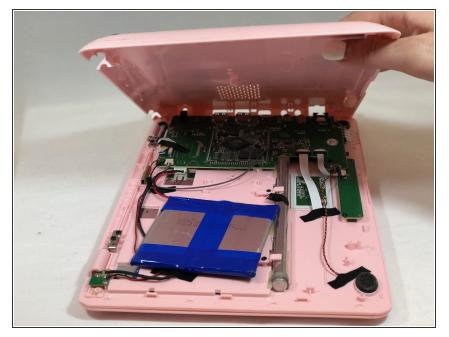
• Remove the bottom of the netbook by lifting the corners.
