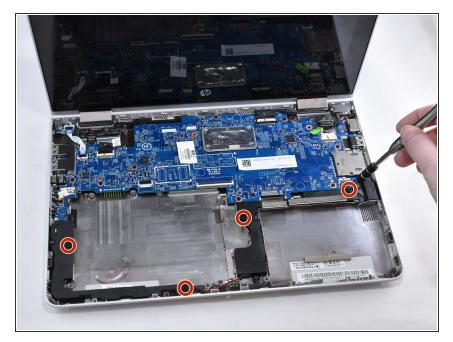
Remove the four 6.2mm Phillips #1 screws around the speakers.
