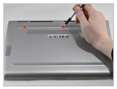
Remove the three 5.7mm Phillips #1 screws.
