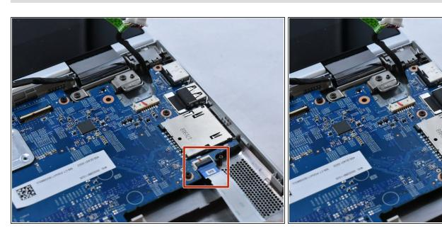
Using your fingernail, disconnect the ZIF (zero insertion force) hard drive cable by flipping up the small locking flap.
