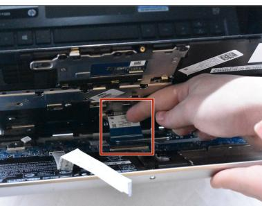
Using your fingernail, disconnect the zero insertion force (ZIF) connector for the touch pad cable by flipping up the small locking flap.
