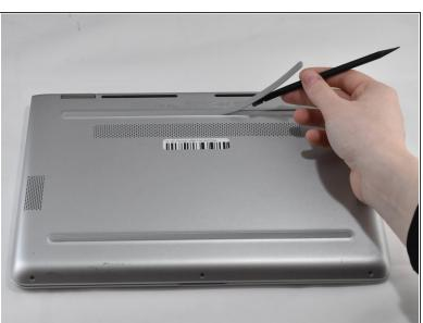
Using a plastic spudger, remove the grey silicon strip closest to the back-side.
