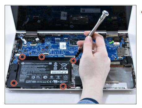
Remove the five 4.6mm Phillips #1 screws located around the battery.
