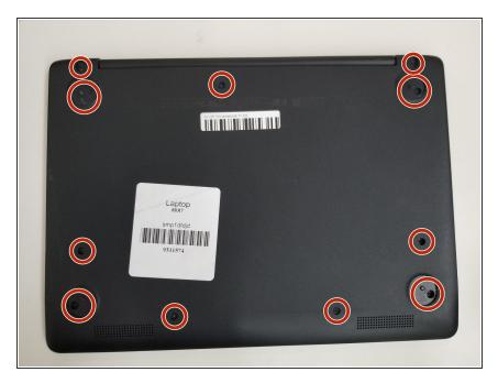
Remove the 4mm eleven screws using a Phillips #00 screwdriver.
