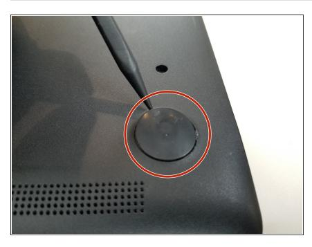
Remove four large rubber pads from the bottom of the device to reveal screws using the pointed end of a spudger.
