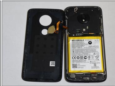
Use the iFixit pick and the iFixit opening tool to pull the fingerprint scanner off of the back case.
