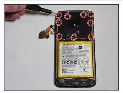
Remove the nine 3.2mm screws from the motherboard cover with a Phillips #00 screwdriver.
