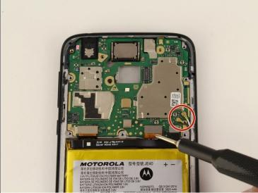
Once the motherboard cover is removed, disconnect the four ribbon cables and the two wires attached to the motherboard.
