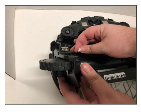
Disconnect the wire carefully from the wheel assembly by pinching and pulling away from it.
