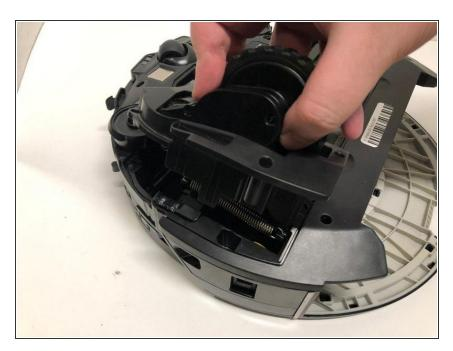
Carefully lift the wheel assembly out of the housing, making sure not to damage its connecting wire.
