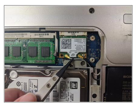
Using a pair of tweezers, remove the two wires as directed.
