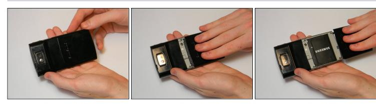
• Apply downward pressure to the top of the battery panel while pulling down to slide it off the phone.
