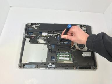
• Using a Phillips #00 screwdriver, remove the seven 1 mm screws.
