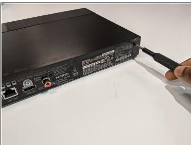
Use the Phillips #2 screwdriver to remove the two 9mm screws located on the back of the device.
