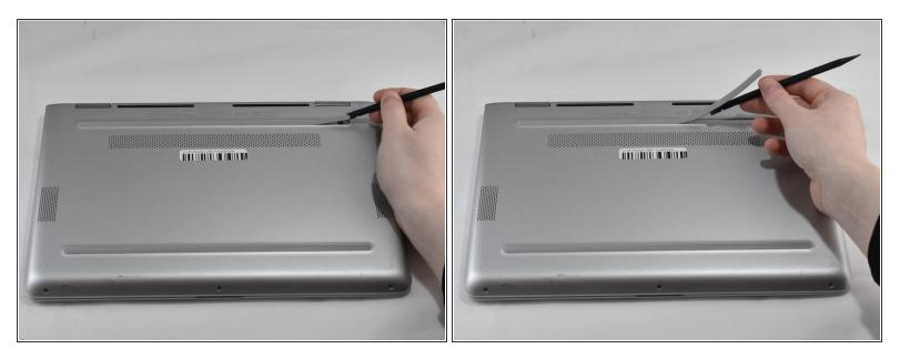
• Using a plastic spudger, remove the grey silicon strip closest to the back-side.
