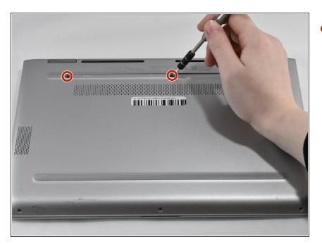
Remove the three 5.7mm Phillips #1 screws.
