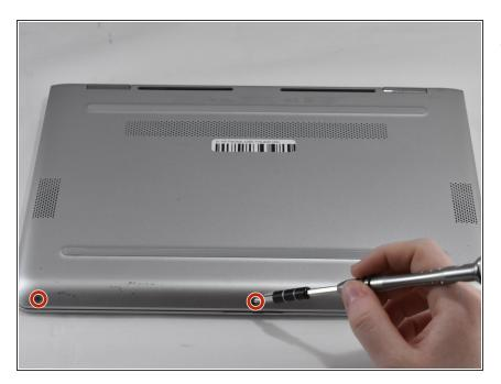
• Remove the three 4.8mm Phillips #0 screws from the front side.
