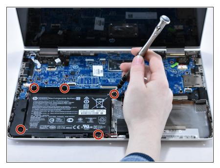
• Remove the five 4.6mm Phillips #1 screws located around the battery.
