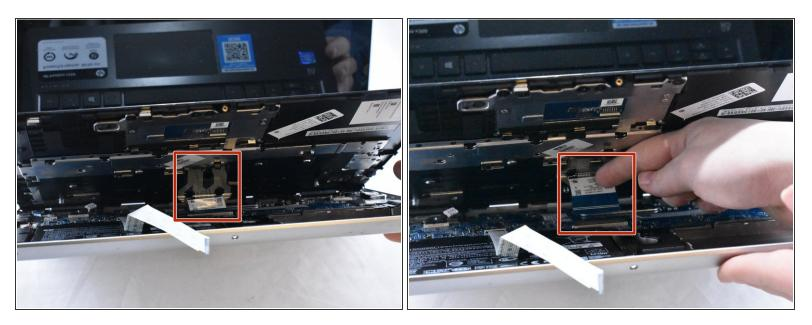
Using your fingernail, disconnect the zero insertion force (ZIF) connector for the touch pad cable by flipping up the small locking flap.
