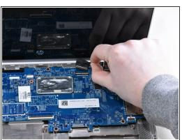
Using your fingernail, disconnect the ZIF display touch screen connector cable from the motherboard.
