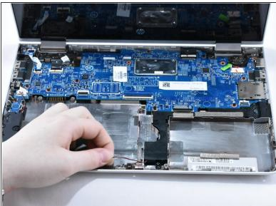
Lift the speaker cable from its retention chamber.
