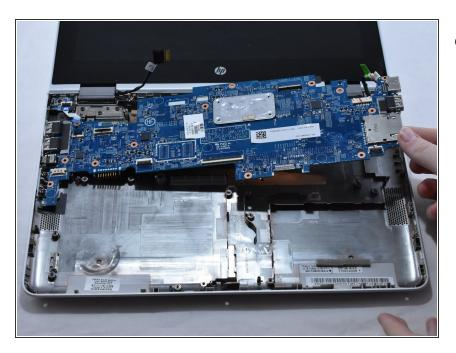
Lift the motherboard up on the right side. Then, gently pull the motherboard straight out to the right.
