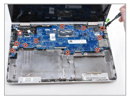
Remove the eleven 4.6 mm Phillips #1 screws from around the motherboard.
