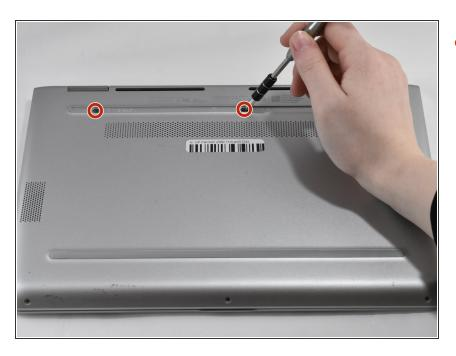
Remove the three 5.7mm Phillips #1 screws.
