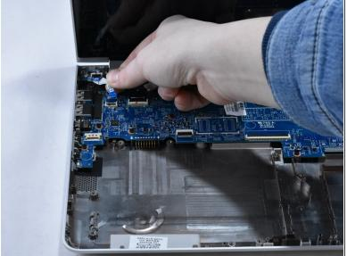
Using your fingernail, disconnect the ZIF (zero insertion force) power button connector cable from the motherboard.
