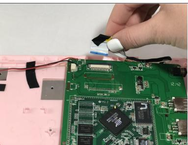
Remove the black covered wire connected to the motherboard by pulling the white ribbon cable away from the motherboard.
