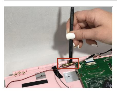
Using a spudger, remove the gold cylinder out of the indent at the bottom of the computer.
