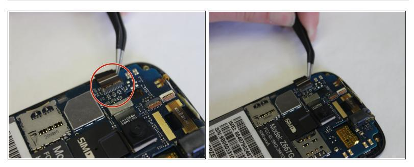
Use a tweezers to lift the lock from the ZIF connector. Pull the ribbon from the connector. (i) Like the camera ribbon, it has a latch that you need to flip to unlock.
