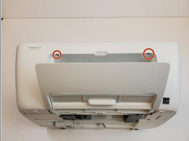
Remove the four screws securing the scanner bed module to the printer body with a Torx T5 screwdriver.
