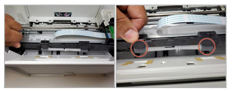
Take a lightly dampened cotton swab and apply it to the grey segments of the rollers.
