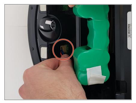
Carefully disconnect the battery cable by pulling near the connector at the bottom of the battery compartment.
