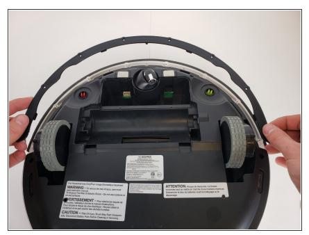
Remove the black strip on the bottom of the bumper.
