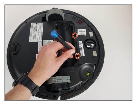
Using a Phillips #0 screwdriver, remove the two 12.25 mm screws holding the battery cover in place.
