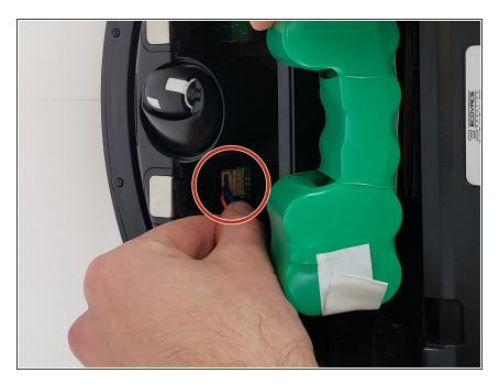
Carefully disconnect the battery cable by pulling near the connector at the bottom of the battery compartment.
