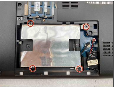
Remove the four Phillips #1 screws from the hard drive bracket.
