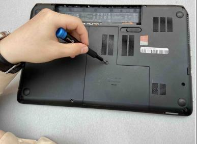
Remove the center screw using a Phillips #1 screwdriver.
