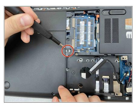
Use a Phillips #1 screwdriver to remove the single screw holding the optical drive
