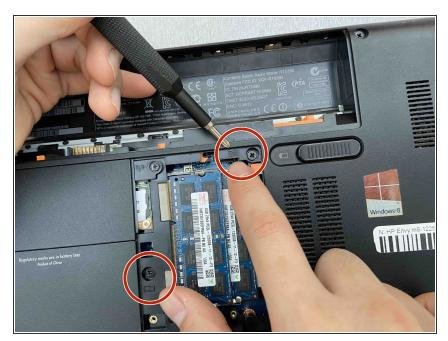
Remove the two Phillips #1 screws that secure the keyboard to the laptop.
