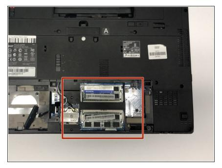
Locate the two RAM sticks on the bottom of the laptop.
