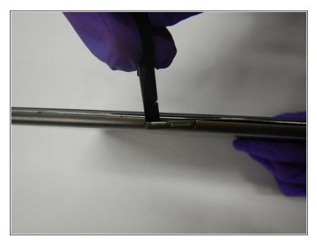
Using a plastic spudger or finger nail, Open the port labeled micro SD using a plastic spudger or finger nail.
