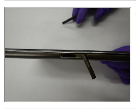
If the SD port is occupied, use a plastic spudger or finger nail gently press the SD card and allow it to protrude.
