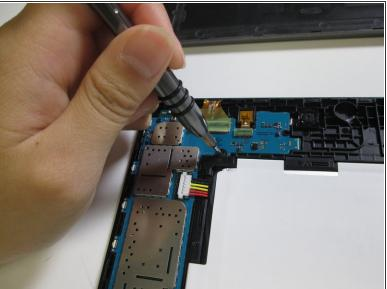
Remove the eleven #000 Phillips 2.8mm screws that hold the battery in place.
