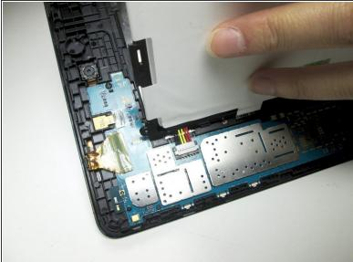
• Pull the battery out until it is only connected to the device by the black, yellow, and red connectors.
