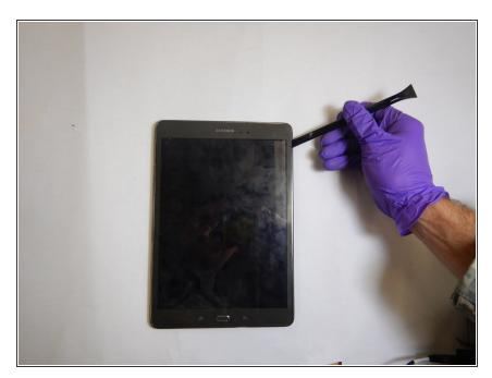
Using a plastic spudger, work around the edge of the screen, prying the screen away from the device.
