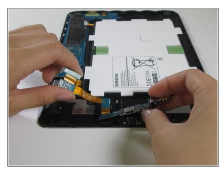
Peel the charging assembly from the device to completely remove the charging port from the device.
