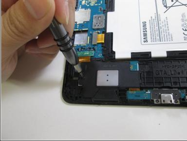
Remove the two 2.8 mm Phillips #000 screws from the speakers.
