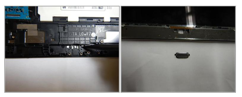
Using the tweezers or a plastic spudger, press on the back of the button until it pops out.
