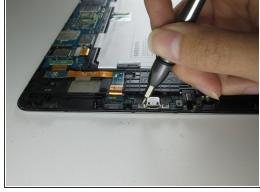
Remove the four 2.8mm #000 Phillips screws that hold the charging port and headphone jack in place.
