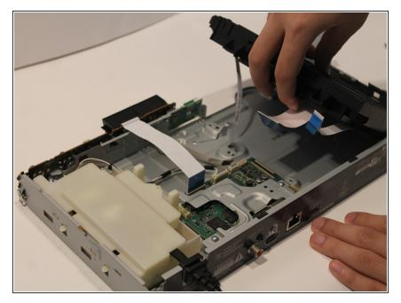
• Remove the metal brace then remove the disk tray.
