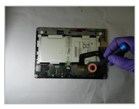
On the right loud speaker, remove 1 screw from the loud speaker module using Phillips #000 screwdriver.
