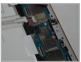
Hold the battery and disconnect the plug to remove the battery.
