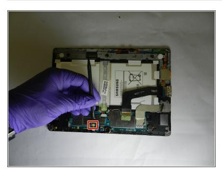
Release the connection of the light sensor, next to the front camera, by lifting up with a spudger.
