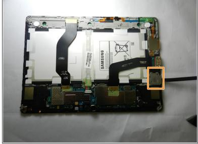
Use a heat gun on the heat bracket and gently pry up the bracket.
