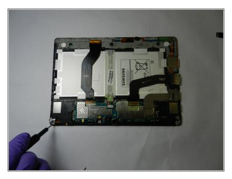
Using the Phillips #00 screwdriver, remove the two screws holding the headphone jack.
