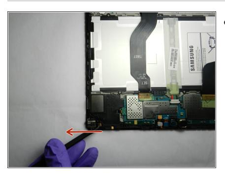
Place the hook of a spudger on the backside of headphone jack and pop the headphone jack out.
