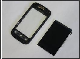
Remove the motherboard to access the screen. Lift the screen away from the front cover and replace.
