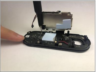
Use the Phillips #000 screwdriver to remove the three screws holding the last circuit board to the black plastic housing.
