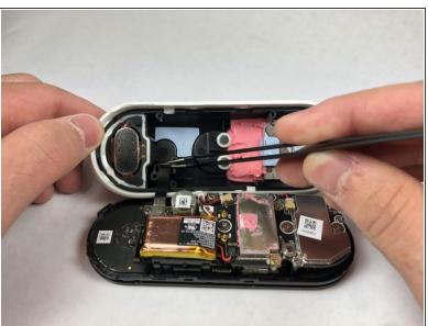
Grip the connector with the tweezers as shown and pull it away from the casing.
