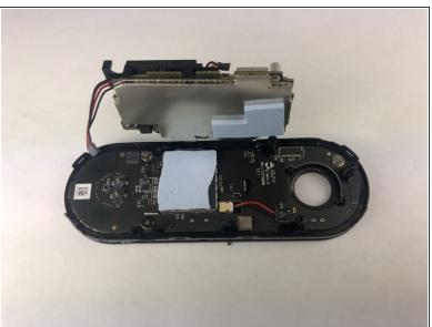
Holding the device as shown push the circuit board away from you and up to free it from the clips.
